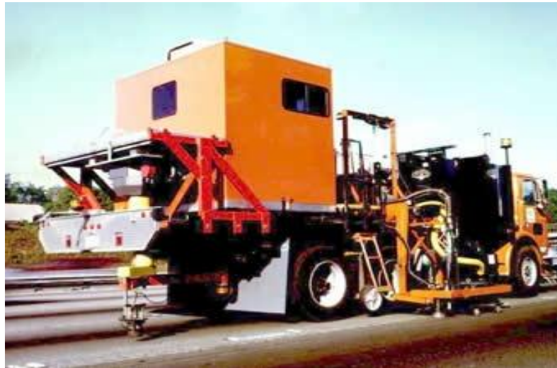
Figure 6. Automated Pavement Crack Sealer
