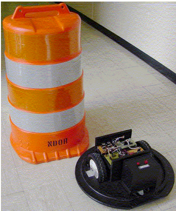
Figure 7. Robotic Highway Safety Marker
